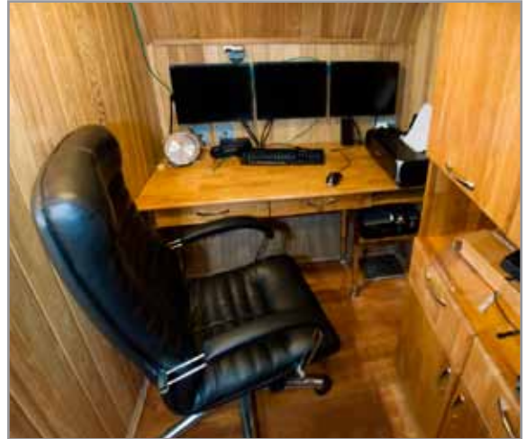
Internal commander console for LSS control.
