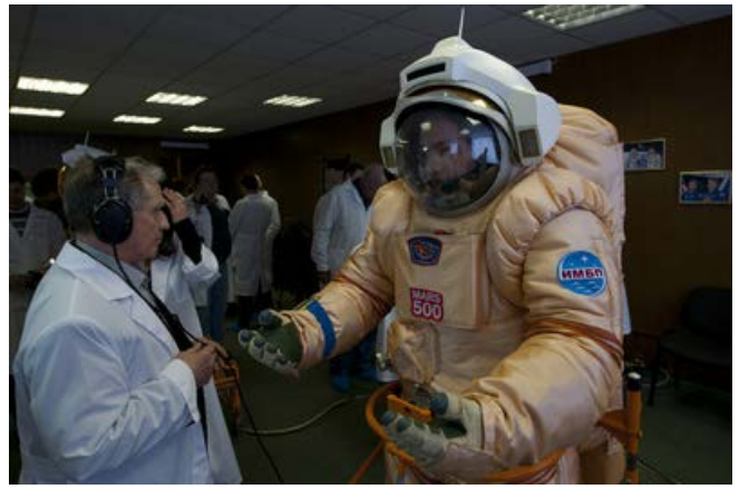
Testing a Martian version of the Orlan spacesuit. Suit has been modified for use in Earth gravity. Credits: ESA/S. Corvaja, 2010
